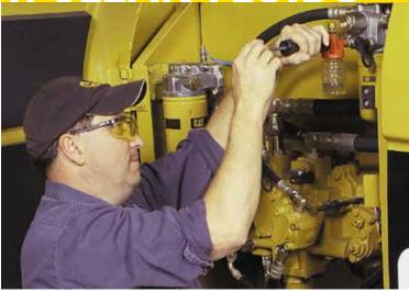
The easiest way for contaminants to enter a system is to enter through "clean" fluids as they go into the machine. Proper fluid handling and clean, tightly sealed containers help prevent this source of potential contamination.
