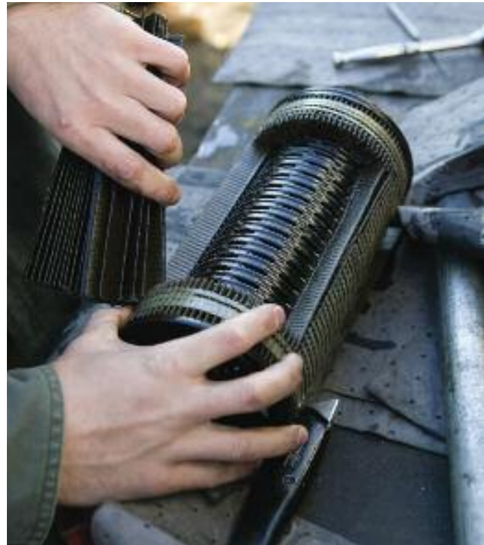
Cutting and inspecting the filters is an important, and telling, aspect of the evaluation.
