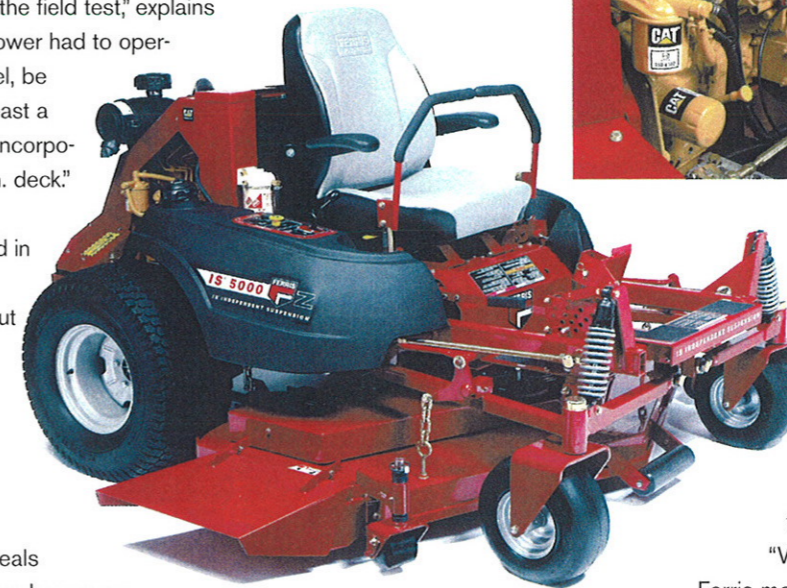
The IS5000Z's 3-cylinder, Cat C1.5 engine provides 31.5 hp with 1,500cc displacement at 2,800 rpm.
