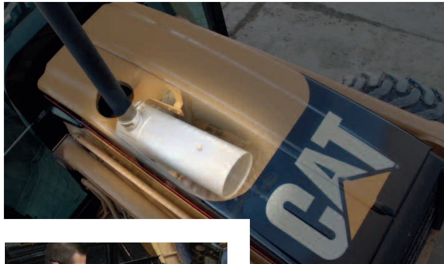
Above: A catalytic converter muffer or “CCM” installed on a backhoe loader.
