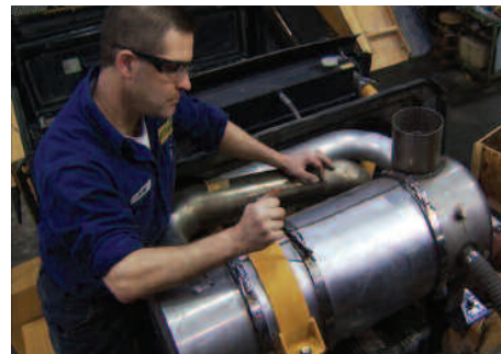
Above: A catalytic converter muffer or “CCM” installed on a backhoe loader.
